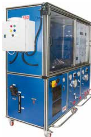
Aerospace Hose Proof & Leak Test Bench for testing hose assemblies to 1000 Bar
